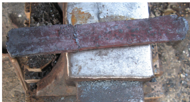
Fig. 4 - Bar hammered from a piece of the bloom
