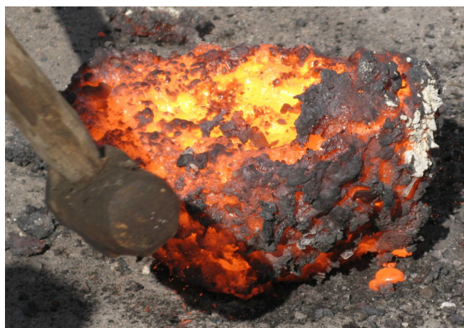
Fig. 3 - Bloom with slag adhering to surface
