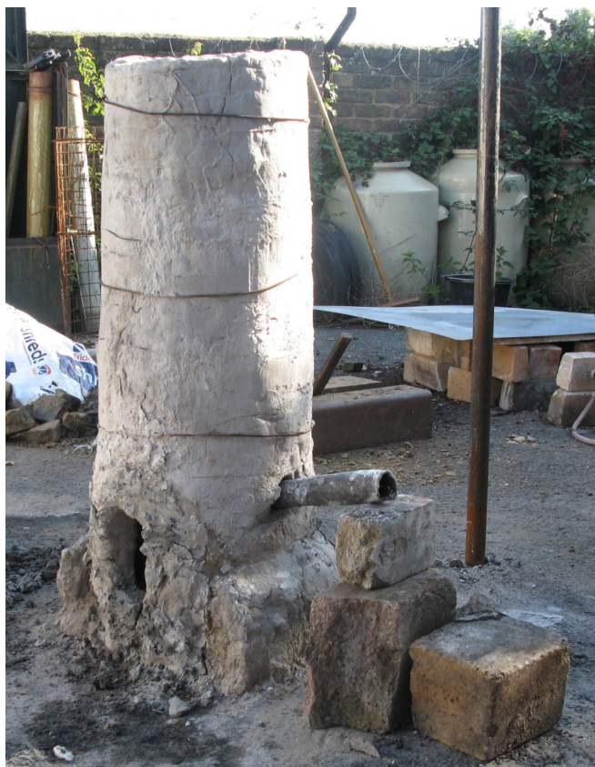
Fig. 1 - Thin walled clay shaft furnace approx 1.5m high and 300mm internal diameter with copper tuyere inclined down 17 deg
