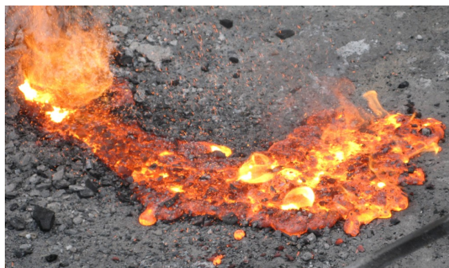
Fig. 2 - Tap slag flowing from 10mm diam hole made in closed slagging arch
