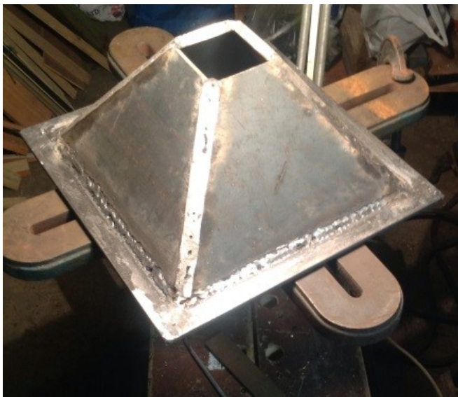
Fig. 2 - The welded sides and flanges...
