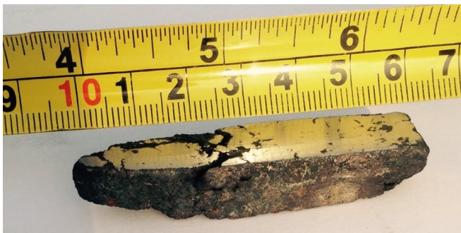
Fig. 9 - The semi-forged bloom
