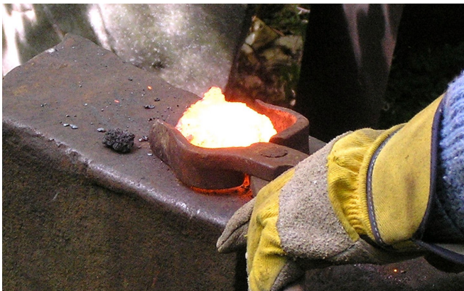
Fig. 8 - Consolidating the bloom
