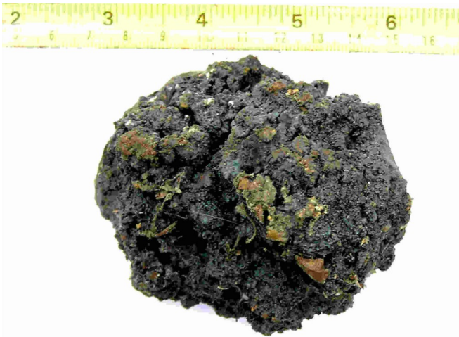
Fig. 7 - The test bloom
