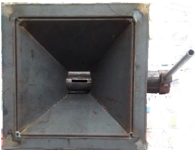
Fig. 4 - The completed forge showing the slotted tuyere background removed
